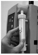
**Figure 6** The humidifier systems of Optiflow and Vapotherm devices.
