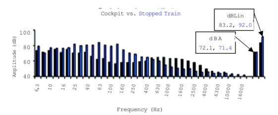
Fig. 2 — Comparison between the frequency distributions obtained within the Airbus-340 cockpit (black) and within an electric commuter train stopped at a station (blue). dBA levels are comparable (72.1 vs. 71.4). dBLin levels are higher than dBA levels: 83.2 vs. 92.0. In both locations, a substantial part of the acoustic energy is concentrated within the lower frequency bands (<500Hz). At the more audible frequencies (>1000 Hz), the amplitude is lower, and above 6300 Hz, it is ≤ 45 dB.
