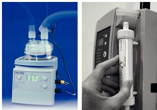
Figure 6 The humidifier systems of Optiflow and Vapotherm devices.
