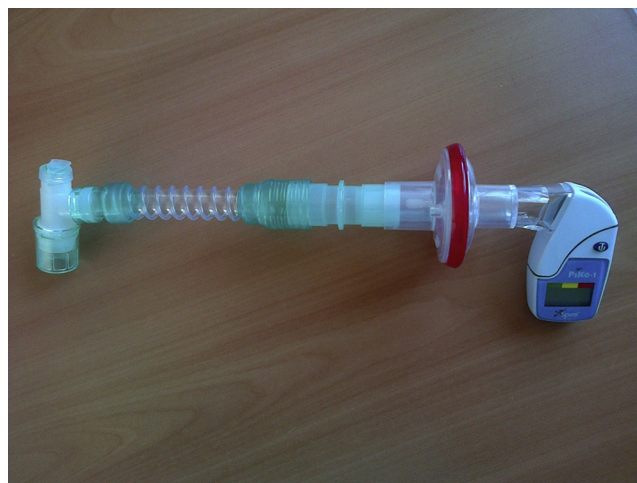
Figure 1 Set-up of an electronic peak flow meter (PiKo I) for measuring cough PEF through the tracheal cannula.
