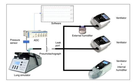
**Figure 1** Simplified scheme of model composition. Every ventilator was connected by means of standard tubing to the lung simulator. Data measured by interposed pneumotachograph and pressure sensor were converted and analysed by specific software. ADC: Analogue to digital converter.
