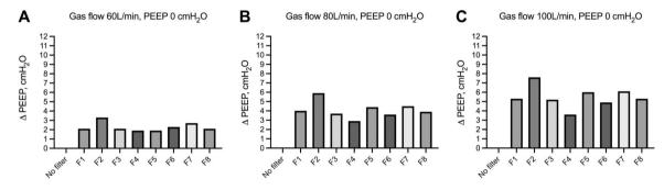
Fig. 2 Change in airway pressure within the hood of the helmet CPAP ( $\Delta$ ZEEP) without and with different HEPA and HMEF filters across increasing gas flows and in the absence of a mechanical PEEP valve. Increasing flow rates are reported in from panel A – 60 L/min; to panel B – 80 L/min; to panel C, 100 L/min. Description of HEPA and HMEF (i.e. from F1 to F8) filters are reported in Table 1. Histobars summarize median and interquartile range.
