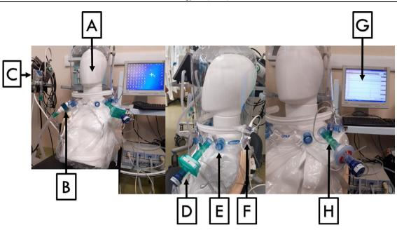
**Fig. 1** Helmet CPAP in vitro configuration. A) Helmet CPAP; B) Pneumotachograph place at the inlet of the helmet; C) Gas flow generator; D) Mechanical PEEP valve with HEPA/HMEF filter; E) Manometer; F) Pressure transducer; G) Acquisition system and pressure and flow tracings; H) airway pressure reading point.
