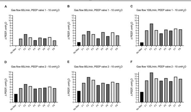
**Fig. 4** Change in airway pressure within the hood of the helmet CPAP ( $\Delta$ PEEP) without and with different HEPA and HMEF filters in presence of mechanical PEEP set at 10 cmH<sub>2</sub>O. Increasing flow rates – from 60 L/min to 100 L/min - are reported in from panel A to panel C by using PEEP valve 1, and from Panel D to panel F by using PEEP valve 2. Description of HEPA and HMEF (i.e from F1 to F8) filters are reported in Table 1. Histobars summarize median and interquartile range.
