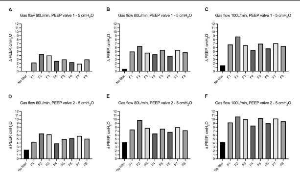
Fig. 3 Change in airway pressure within the hood of the helmet CPAP ( $\Delta$ PEEP) without and with different HEPA and HMEF filters in presence of mechanical PEEP set at 5 cmH<sub>2</sub>O. Increasing flow rates – from 60 L/min to 100 L/min - are reported in from panel A to panel C by using a) PEEP valve 1, and from Panel D to panel F by using PEEP valve 2. Description of HEPA and HMEF (i.e. from F1 to F8) filters are reported in Table 1. Histobars summarize median and interquartile range.
